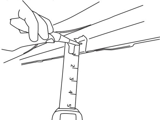
Route LED wires through through grommet, clean surface, and stick on to rocker panel as shown below.
