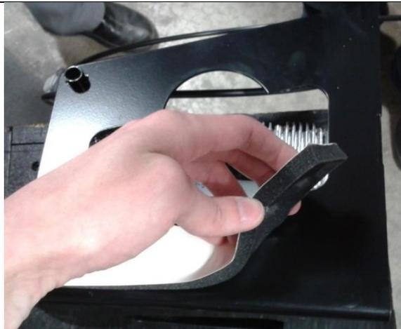
Locate the two mounting points for the compressor. The compressor bracket is designed to line up with the front hood hinge bolt and an existing hole in the inner fender. Remove the hood hinge bolt now to allow for installation of the compressor bracket.
