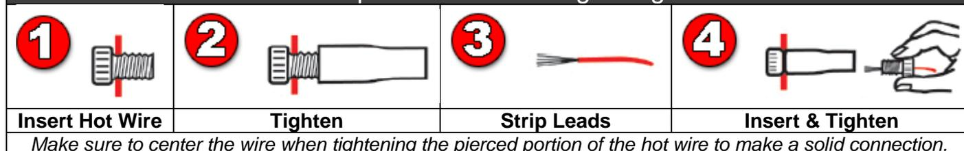
**The ground terminals of the vehicle's batteries should be disconnected before performing any piercing/posi-tapping onto any ECM/PCM wire.**
