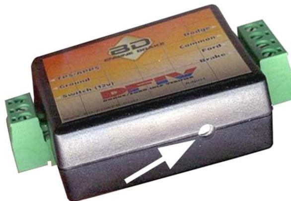
**CAUTION:** THE ADJUSTING SCREW IS A MICRO-SWITCH THAT IS VERY DELICATE, SO TURN USING SMALL ADJUSTMENTS
