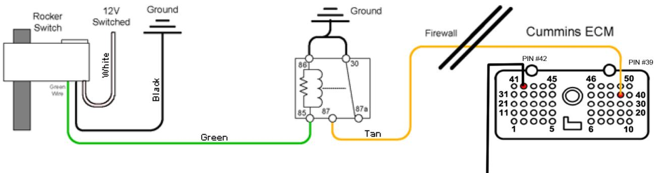
This switch relay is **not required** when wiring the exhaust brake with the push-pull style switch.
