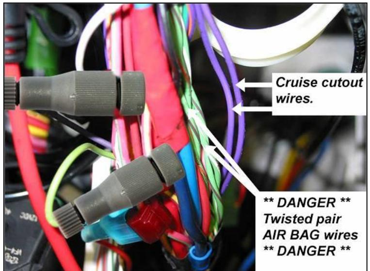
In this same wiring harness, locate the **violet w/ Brown tracer** wire and install another gray Posi-Tap. Insert the **green** wire from the “Com” terminal of the DFIV module into this connector.
