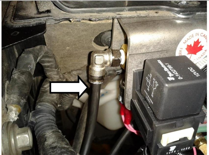
The other line of the compressor is the air suction line. This line is a 1/4" diameter and comes with a preinstalled threaded adapter. Install the threaded filter supplied with the air pump into this fitting.
