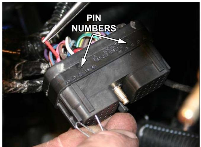
The two wire leads from the exhaust brake control harness (with the ECM pins pre-crimped) can now be plugged into the ECM. Insert the tan wire into Pin #39, and the black wire to Pin #42. They should snap into place. Once this is complete, you can re-install the ECM plug. Secure the wiring loom using the supplied tie wraps.
