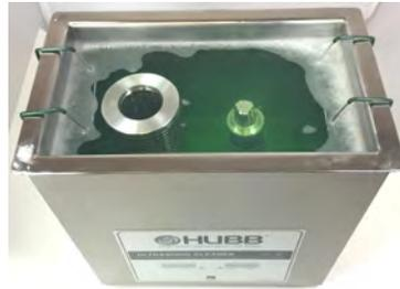
5. Press ON/OFF to begin the cleaning cycle. Once cleaning cycle is complete, the cleaning station will automatically shut off.
