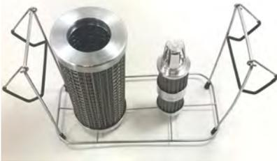
2. Place rack with filters in to cleaning station
