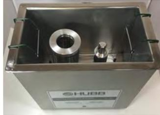
3. Add correct measured amount of HUBB Cleaning Concentrate to Cleaning Station.
