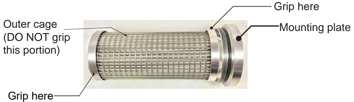
In this situation, grip the primary filter media assembly by the base (do not grip the filter by the outer cage) carefully unscrew the primary filter media assembly from the mounting plate (turning counterclockwise).
